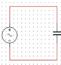
Figura 49 –  $Z_2 = 10\angle -90^\circ\Omega$
