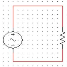
Figura 48 –  $Z_1 = R = 10\Omega = 10\angle 0^\circ\Omega$
