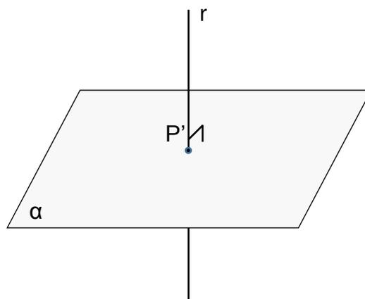
$$\begin{aligned} r &\perp \alpha \\ r \cap \alpha &= P' \\ P' &= \text{proj}_{\alpha} r \end{aligned}$$
