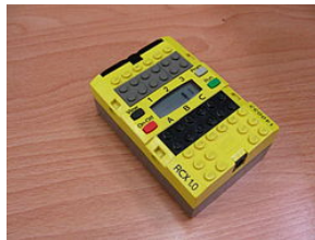
Figura 3.12: RCX - Robotic Command Explorer - Controlador Fonte: https://legoways.com/lego-mindstorms-buyer-guide/
