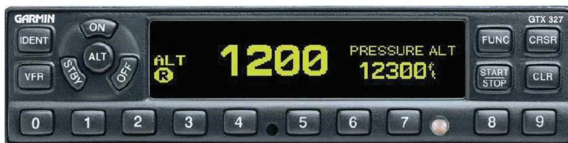
Figura 19 – Painel de controle do Transponder
