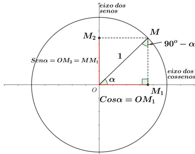
Figura 1.8: seno de  $\alpha$  e cosseno de  $\alpha$ , com  $0 \leq \alpha \leq 2\pi$
