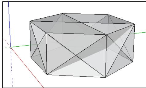
Figura 42 - Marcando centro das faces do prisma hexagonal regular
